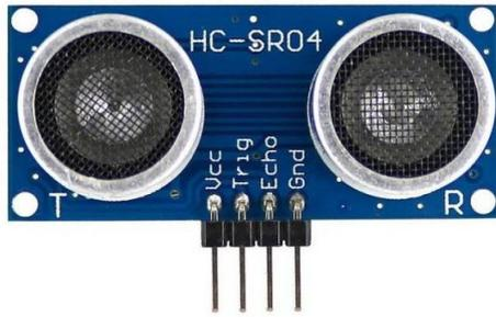
Figure 3. Ultrasonic Sensor
