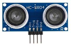
Figure 3. Ultrasonic Sensor
