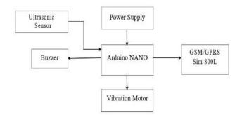
Figure 1. Block Diagram
