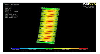
Fig.3 Deflection and shear stress contour for square cross section helical spring for Length 150 mm
