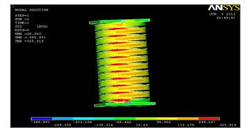
Fig.4 Deflection and shear stress contour for square cross section helical spring for Length 125 mm
