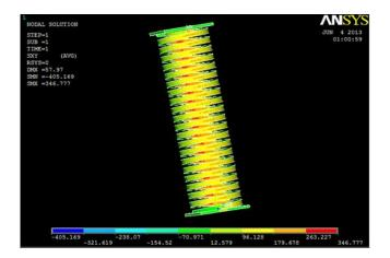
Fig.6 Deflection and shear stress contour for rectangular cross section helical spring for Length 225 mm (B = 1.5 H)
