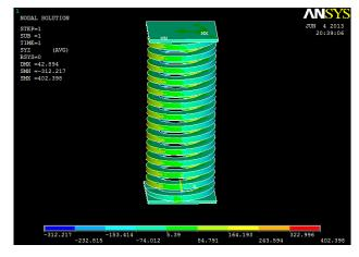
Fig.13 Deflection and shear stress contour for rectangular cross section helical spring for Length 150 mm (B = 2 H)
