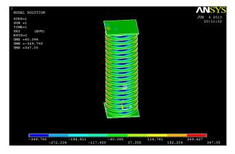
Fig.12 Deflection and shear stress contour for rectangular cross section helical spring for Length 200 mm (B = 2 H)
