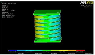
Fig.5 Deflection and shear stress contour for square cross section helical spring for Length 75 mm
