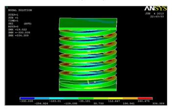
Fig.15 Deflection and shear stress contour for rectangular cross section helical spring for Length 75 mm (B = 2 H)
