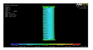
Fig.1 Deflection and shear stress contour for square cross section helical spring for Length 225 mm
