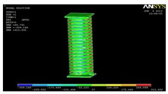
Fig.2 Deflection and shear stress contour for square cross section helical spring for length 200 mm
