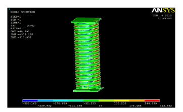
Fig.7 Deflection and shear stress contour for rectangular cross section helical spring for Length 200 mm (B = 1.5 H)
