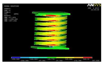
Fig.10 Deflection and shear stress contour for rectangular cross section helical spring for Length 75 mm (B = 1.5 H)
