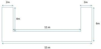
Fig 1: Schematic diagram of the hearth used in the study
