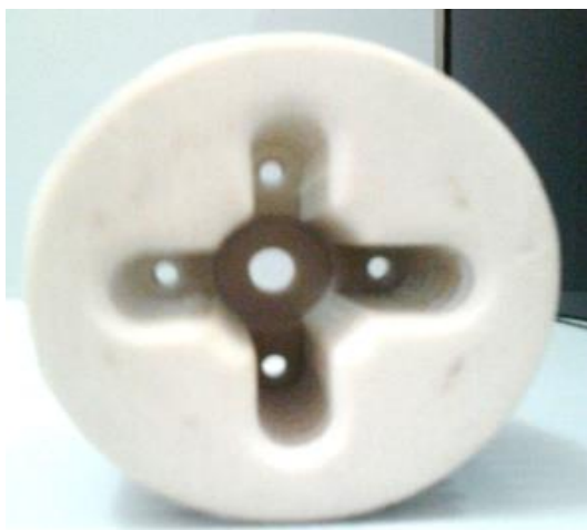
Fig 12 Final Manufactured Cooling Head
