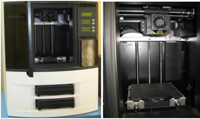
Fig. 5 Fused Deposition modelling (Machine)
