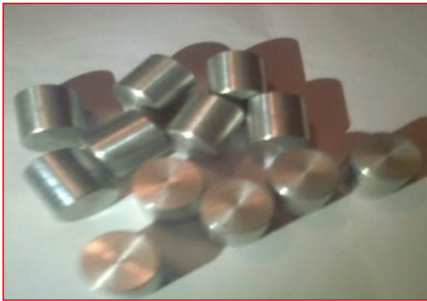
Fig. 6 Corrosion test specimens
