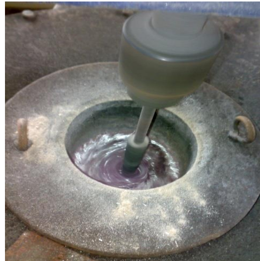
Fig. 3 Mechanical Stirrer in action
