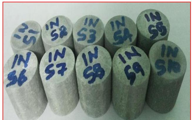
Fig. 9 Corrosion Test Specimens
