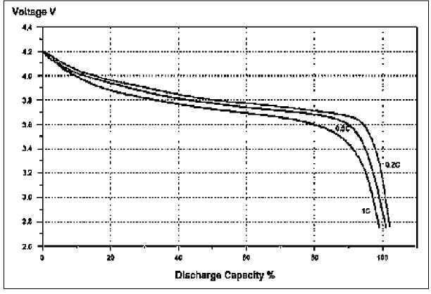
Figure 6 – Voltage vs. Discharge Capacity at Different C – Rates
