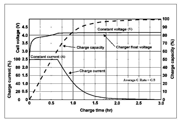
Figure 5 – Charging Characteristics for C – Rate of C/3
