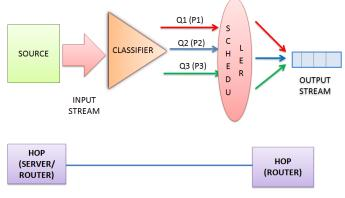
Figure 1 : Architecture of Hybrid FQ-CoDel
