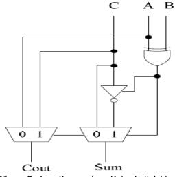
Figure 7 : Low Power – Low Delay Full Adder
