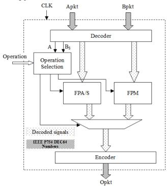
Figure 2 : High Level Block diagram – Floating point Unit
