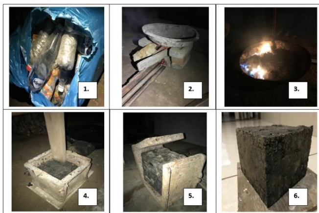
Fig 3:- 1) Weighed plastic, 2) Heating set-up, 3)Addition of plastics into the heated set-up, 4)Casting, 5)Drying and Molding, 6)Block
