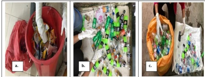
Fig 2:- a) Collection of plastic waste from institutional dustbins, b)Washing and Drying of plastics, c)Storage of plastic waste (PET plastic bottles)
