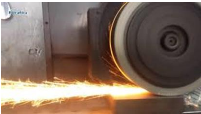
Fig: 3.5. Grinding operation
