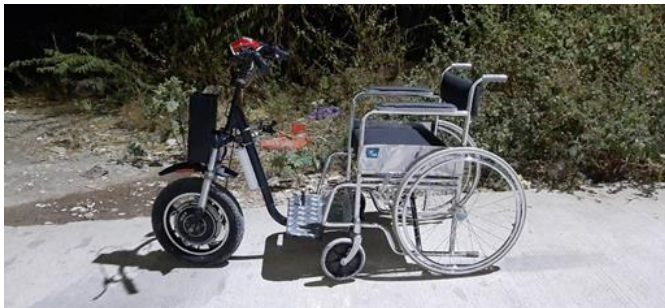
Fig: 4.1. Final model of automated wheel chair
