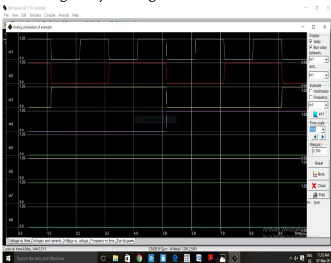
Fig 9 :Voltage Vs Time of 12T SRAM Cell
