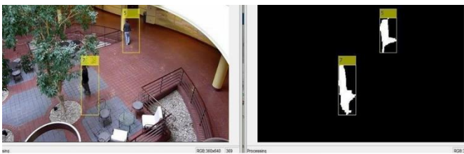
Fig 5: Input Normal video fig 6: Output Gaussian models
