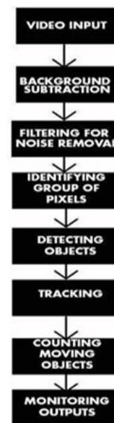
Fig 2: Flow of Operation
