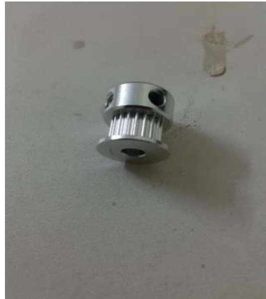
Figure 5(a) - GT2 pulley
