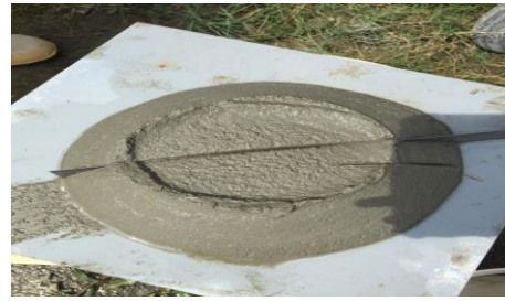
Fig 4 : Slump Flow Trial Harden Characteristic Trial
