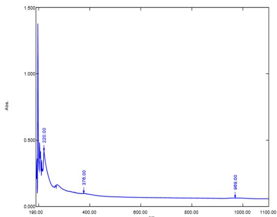
Figure 3: Absorption Spectrum of ZnO nanoparticles calcined at 400° C
