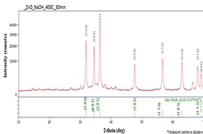
Figure 1: ZnO Nanoparticles calcined at  $400^\circ\text{C}$ .
