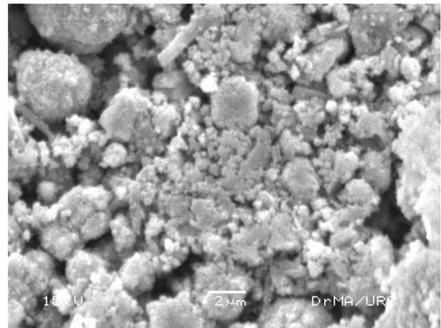
Figure2: SEM image of ZnO Nanoparticles calcined at 400 °C
