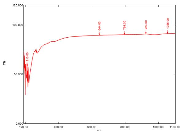
Figure 4: Transmittance Spectrum of ZnO nanoparticles calcined at 400° C .
