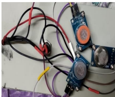
Fig-3 : Electronic device gas sensing system.
