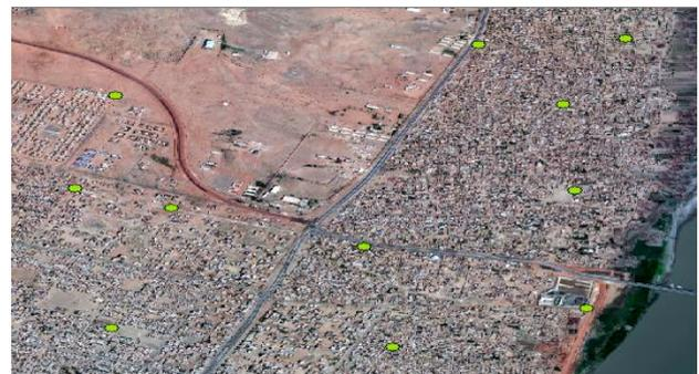
**Figure 9 :** Ten Distribution Control Points and Check Point
