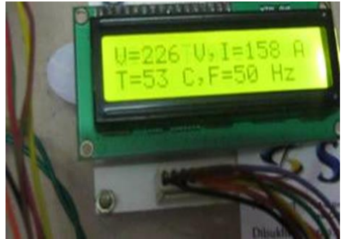
Fig 8 - Actual Electrical Parameters Such as Current, Voltage, Frequency and Temperature recorded as OutputAC
