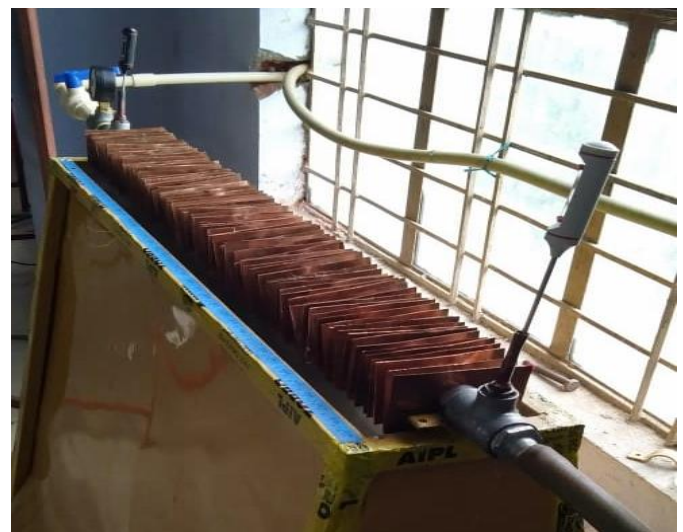
Figure 5 : Physical setup for heat exchanger with spiral grooving with rectangular copper fin.
