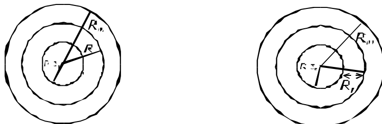
Fig. 7(a) cross-sectional view of the nanorod before melting of shell Fig. 7(b) cross-sectional view of the cylinder on melting of shell
