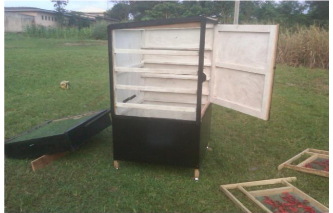
Figure 3.2 : Drying cabinet with the tilted solar collector
