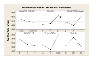
Figure 8: Main effect plots of TWR for H11 workpiece
