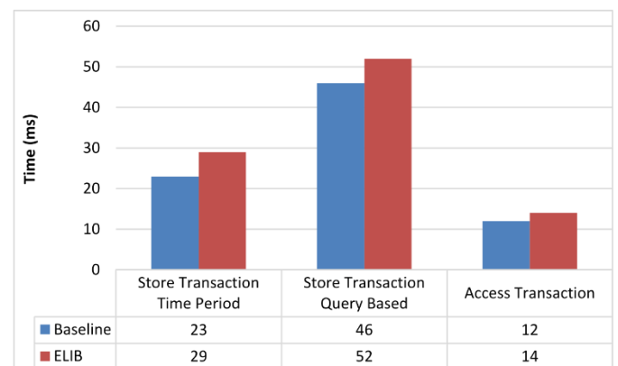
Fig. 5. Evaluation of time overhead in the LBM.
