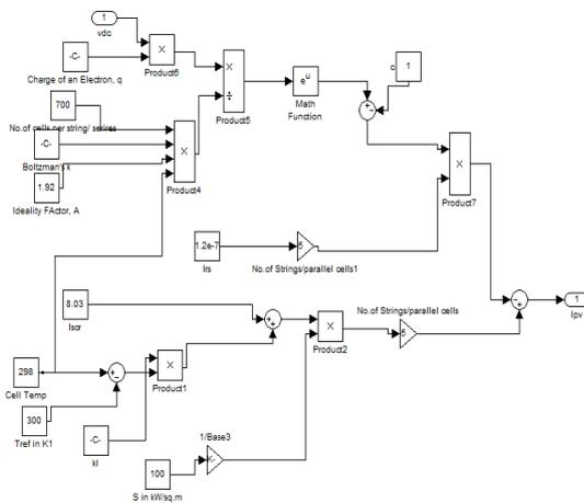
**Figure 4 :** Unmasked block diagram of the modeled solar PV panel
