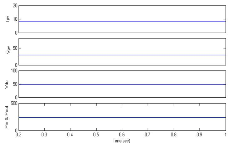
**Figure 6 :** Steady State Performance of Standalone PV based boost converter
