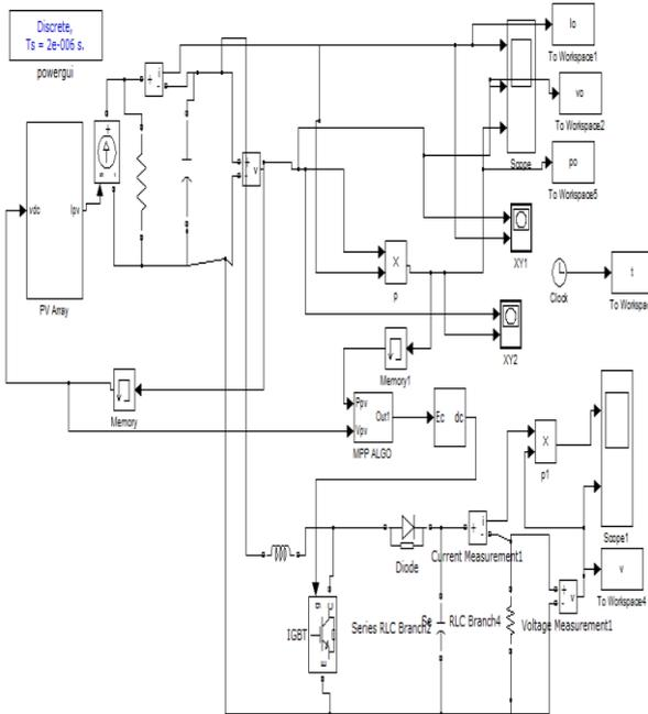
**Figure 3:** MATLAB simulated modal of PV based boost converter
