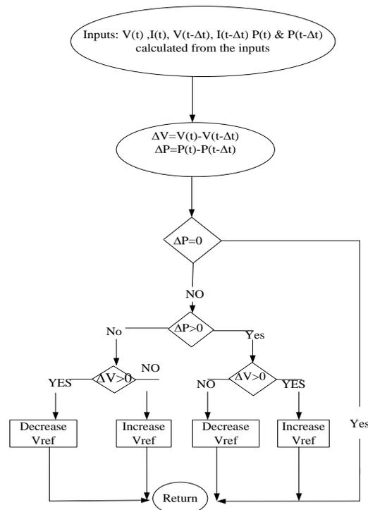
Figure 2 : Flowchart of Perturb & Observe algorithm
