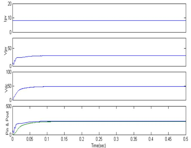
**Figure 5 :** Starting performance of standalone PV based boost converter
