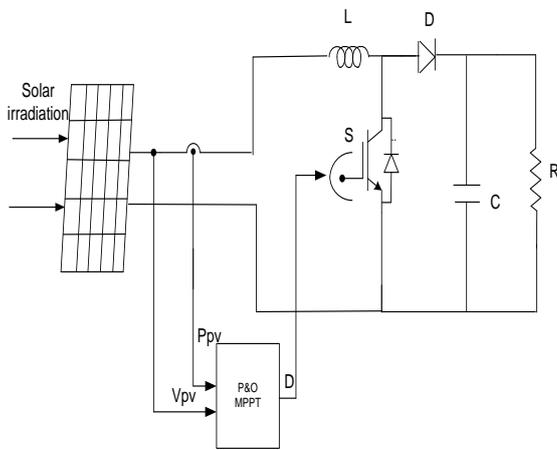
Figure 1 : PV based Boost converter
