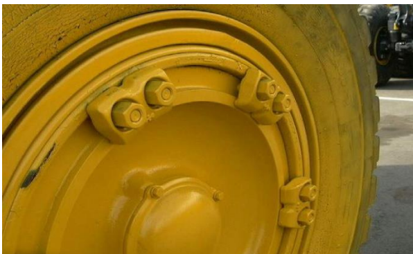
Figure 2. Wedge type wheel/rim on the dump truck
