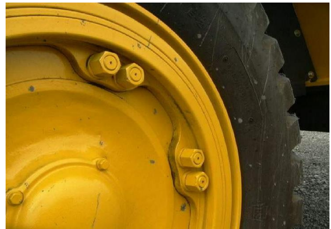
Figure 3. Disc wheel/rim mounted on the dump truck
