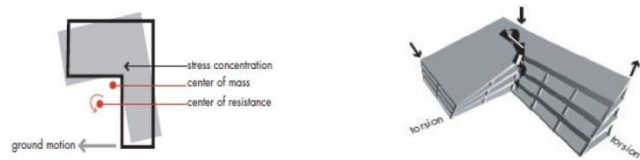
Fig 4: Damage at re-entrant corner in L-shaped buildings
