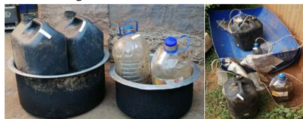
Figure 2 : Large-scale biogas production from pretreated market wastes
