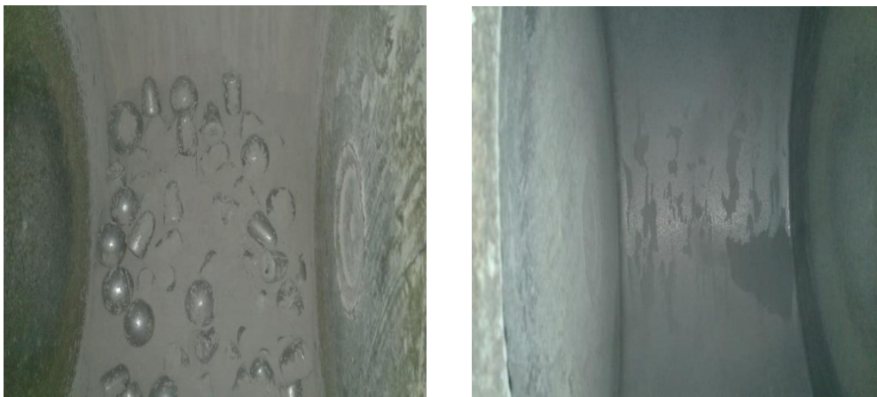
Fig. 6. Photos taken at the opening of the mill and after discharging the fine grinded mixture of ETP slag with fly ash
