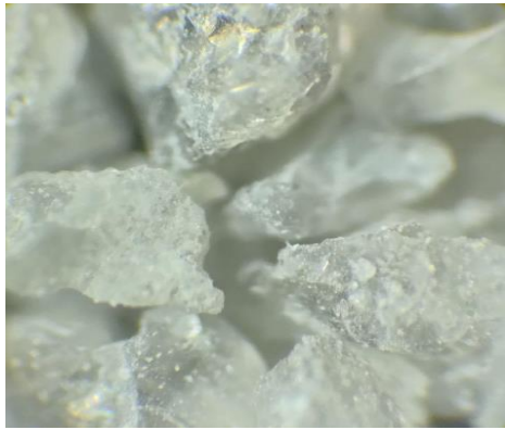
Fig. 2. Macro- and microphotographs of granulated ETP slag (x 120 times)
