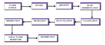
Figure 3 : Flowchart –Water Treatment Plant
