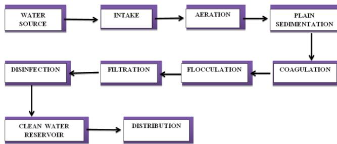
Figure 3 : Flowchart –Water Treatment Plant
