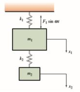
Figure 1 : Two DoFUndamped Dynamic Vibration Absorber
