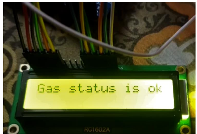
Fig 12. : LCD showing output of no gas leakage.
