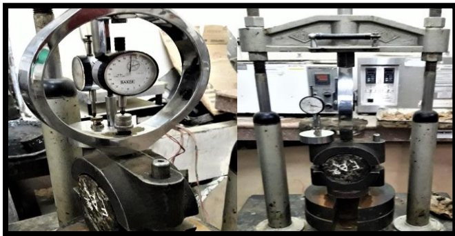
Sample testing on Marshall Stability machine
