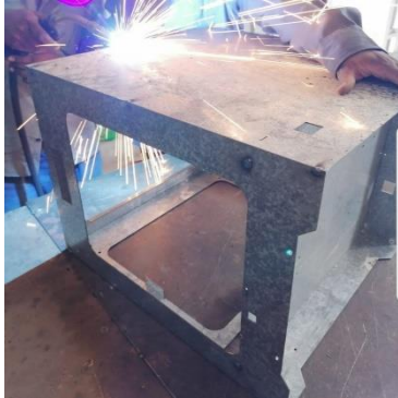
Figure 3: Welding Process of Machine Frame
