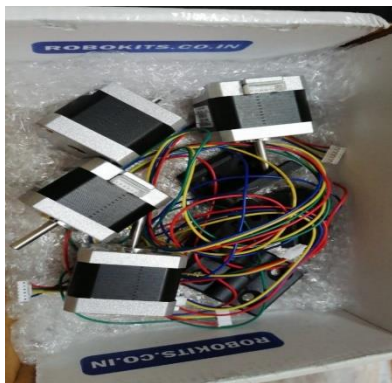
Figure 4: Stepped motors used in machine
