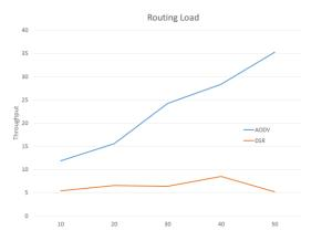
Figure 4: Comparison of AODV and DSR Routing Lode
