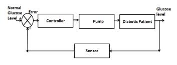
Figure 1 : Block diagram of Glucose Insulin regulation system<sup>[3]</sup>
