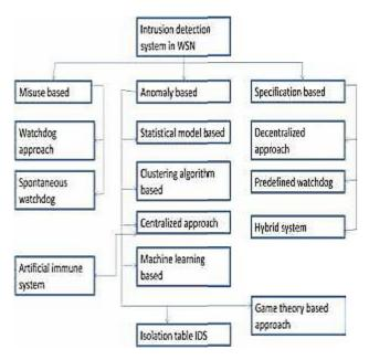
**Figure 2 :** Taxonomy of Intrusion Detection Systems in WSN
