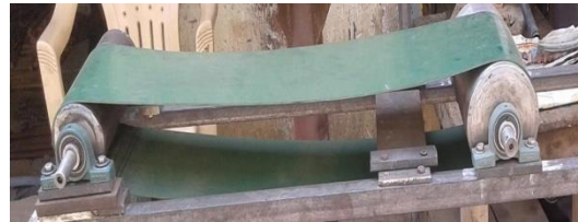
Fig.14 Fabricated roller with conveyor
