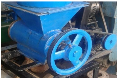
Fig.21 Fabricated screw feeder cylinder with dropbox
