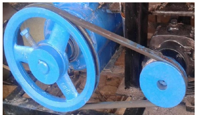
Fig.18 Fabricated pulley arrangement for screw feeder and reduction gearbox with v belt
