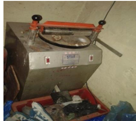
Fig.2 Semi-automatic rotli making machine with single roller and supporting plate
