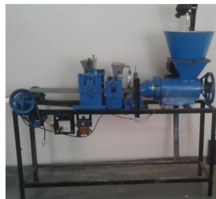
Fig.23 Unbaked rotti making machine
