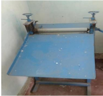
Fig.1 Semi-automatic portable unbaked rotli making machine
