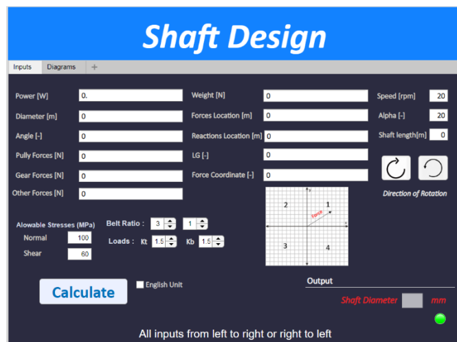
Figure (2) Proposed Shaft design GUI
