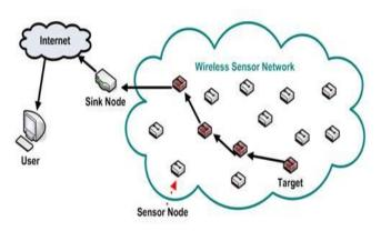
Figure 1: Architecture of a Wireless Sensor Network
