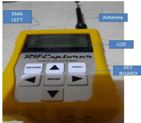
Figure 2.8 : RF Explorer Spectrum Analyzer
