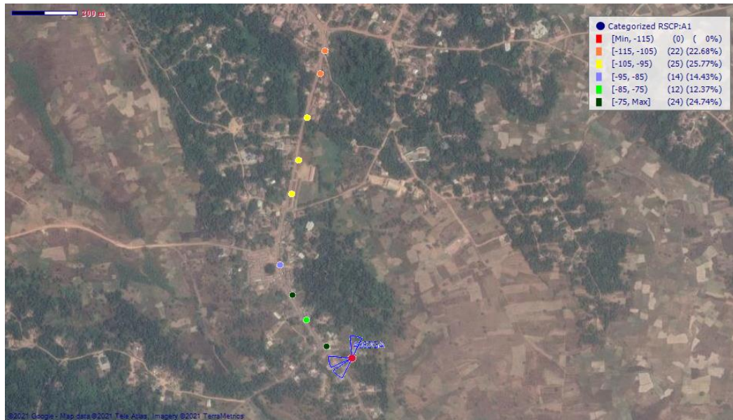
Figure 2.3 : Pathloss Propagation towards Renaissance University from the computer screen
