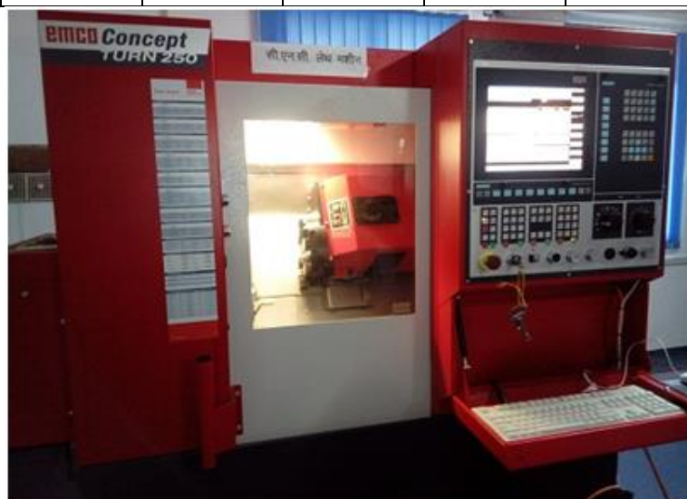
Figure 1: Photograph of EMCO Concept Turn 250 machine tool used for turning.
