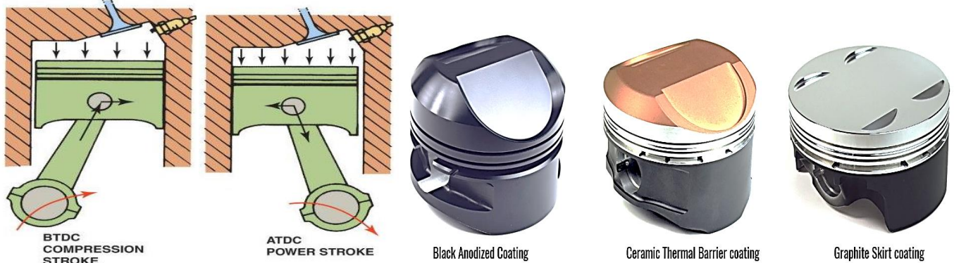
Fig 2. Different types of piston coatings
