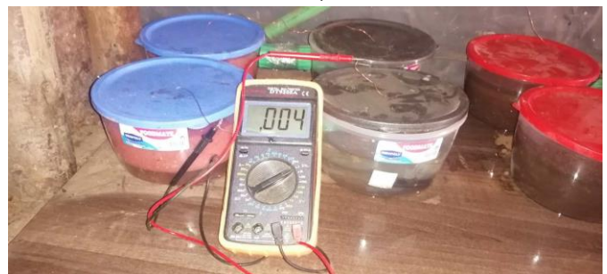
Figure 4 : Set-up of H-shaped microbial fuel cells with a multi-meter
