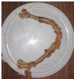
Figure 2: Salt bridge prepared wicks, 3% agarose in NaCl
