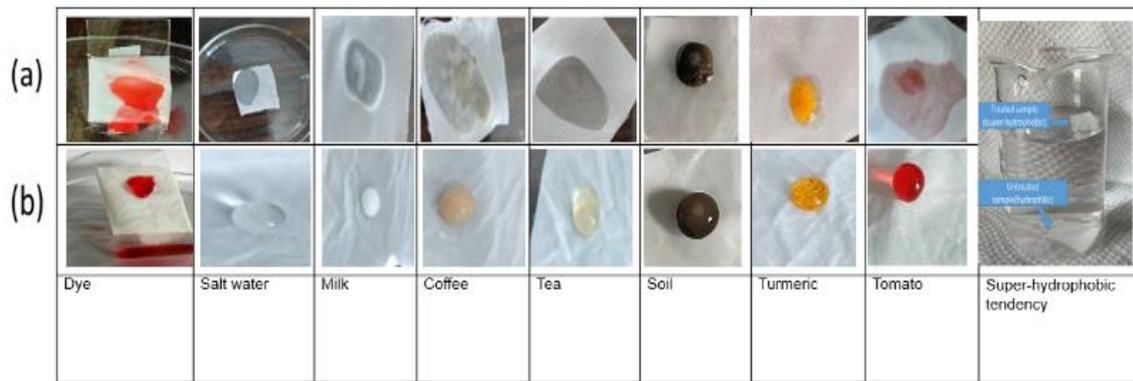
Figure 12 : Comparison of Cleaning tendency by using dye, salt-water, milk, coffee, tea, soil, turmeric and tomato solution (a) untreated sample,(b)treated sample and floating tendency of super-hydrophobic treated sample.
