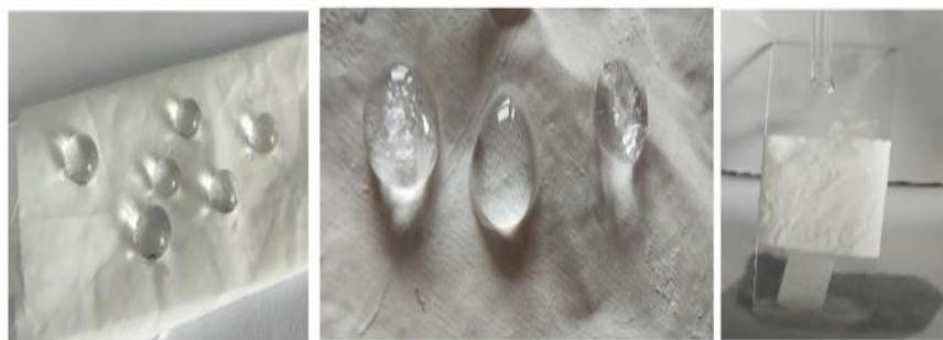
Figure 12 : (a) Frozen water on the treated surface of the static test, (b) frozen water after 3s, (c) dynamic condition of de-icing test with super-cooled water.
