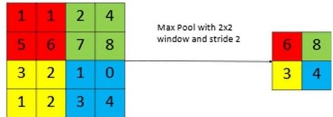
Fig 3: Max pool Operation in CNN [16].
