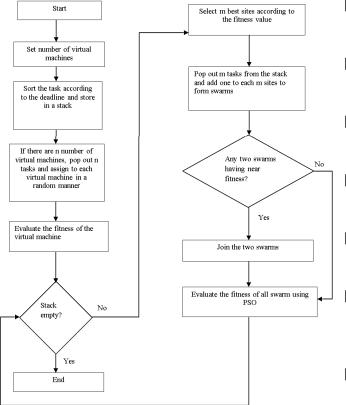
Figure 1 : Flow chart of the HBPSO algorithm for task scheduling and resource allocation
