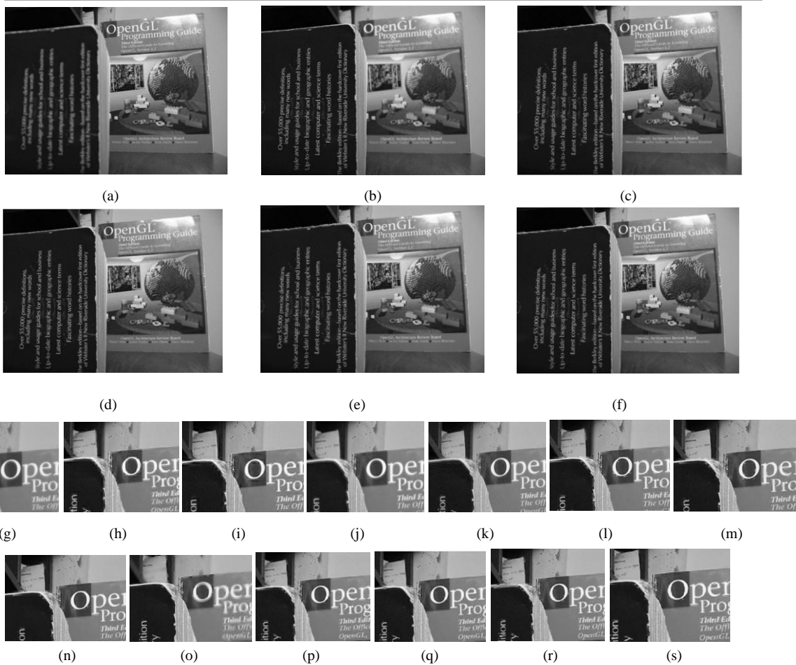
Figure 5. Source images "Book" and fusion results. (a) First source image with focus on the right. (b) Second source image with focus on the left. (c) DCT + EOL (proposed) result. (d) DCT+VOL(proposed). (e) DCT+Corr(proposed). (f) DCT+Eng_Corr (proposed). (g), (h), (i), (j), (k), (l), (m), (n), (o), (p), (q), (r), and (s) are the local magnified versions of DCT+Average, DCT+Contrast, DWT, SIDWT, DCHWT, DCT+Variance, DCT+Ac_Max, DCT+SF, DCT+SML, DCT+EOL(proposed), DCT+VOL(proposed), DCT+Corr(proposed), and DCT+Eng_Corr (proposed), respectively.
