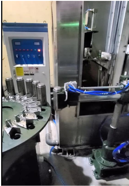
Figure 8. Robot picks up workpiece in heating machine to the collection table
