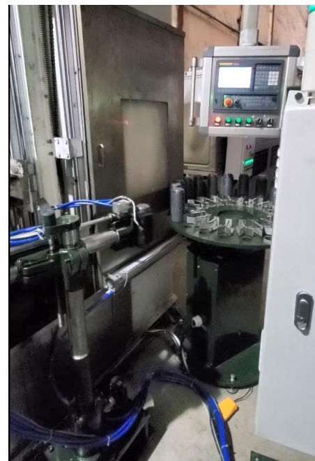
Figure 7. Robot picks up workpiece from the feeder table
