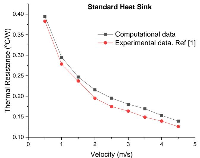
Figure 5: Validation with respect to Thermal Resistance
