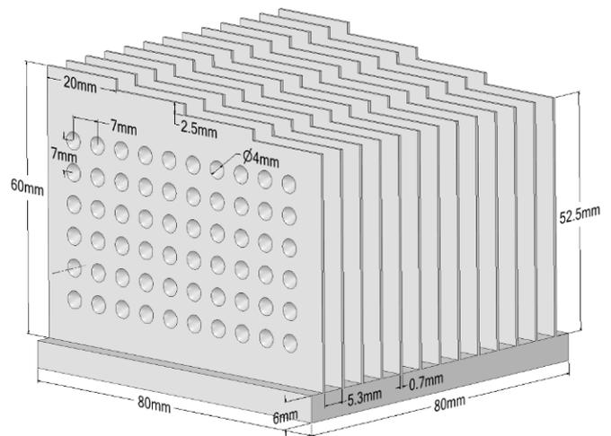
Figure 2: Stepped flat plate HS with inline dimples
