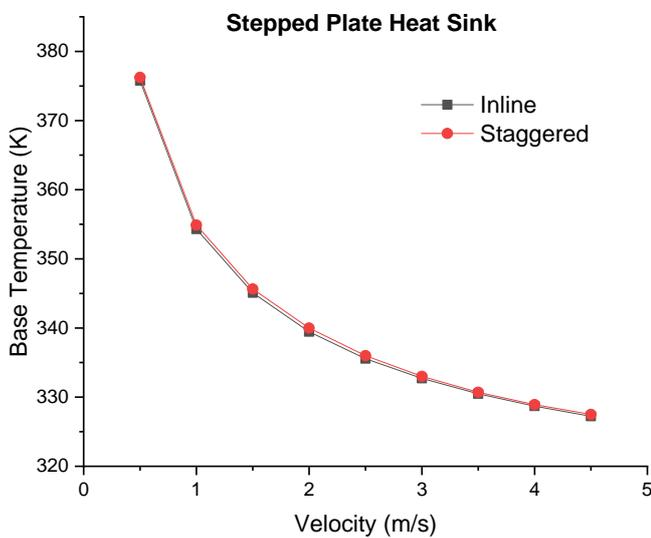
Figure 10: Variation of base temperature with velocity
