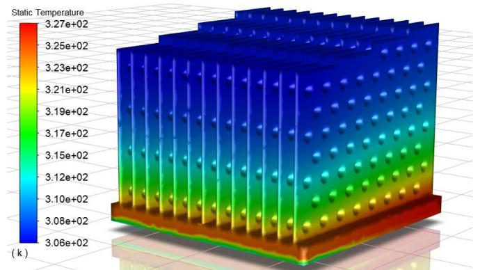
Figure 9: Base Temperature contours of staggered dimpled HS at 4.5 m/s
