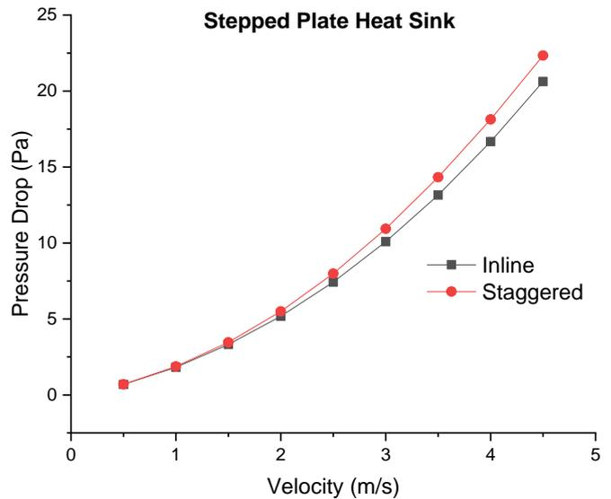
Figure 11: Variation of pressure drop with velocity
