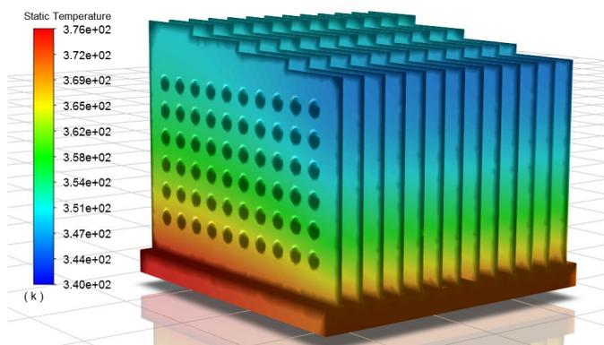
Figure 6: Base Temperature contours of inline dimpled HS at 0.5 m/s
