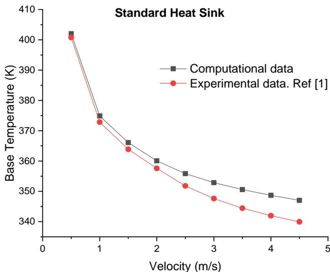
Figure 4: Validation with respect to Base Temperature
