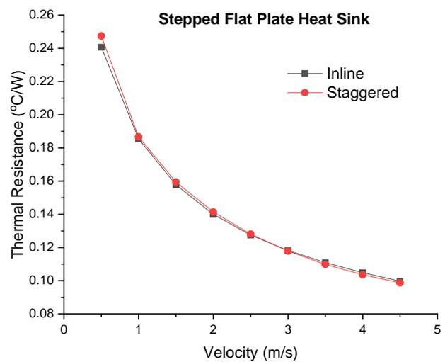
Figure 12: Variation of thermal resistance with velocity
