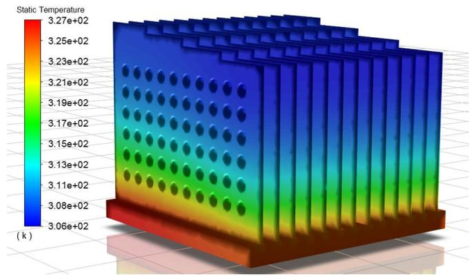
Figure 8: Base Temperature contours of inline dimpled HS at 4.5 m/s
