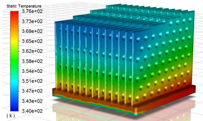
Figure 7: Base Temperature contours of staggered dimpled HS at 0.5 m/s
