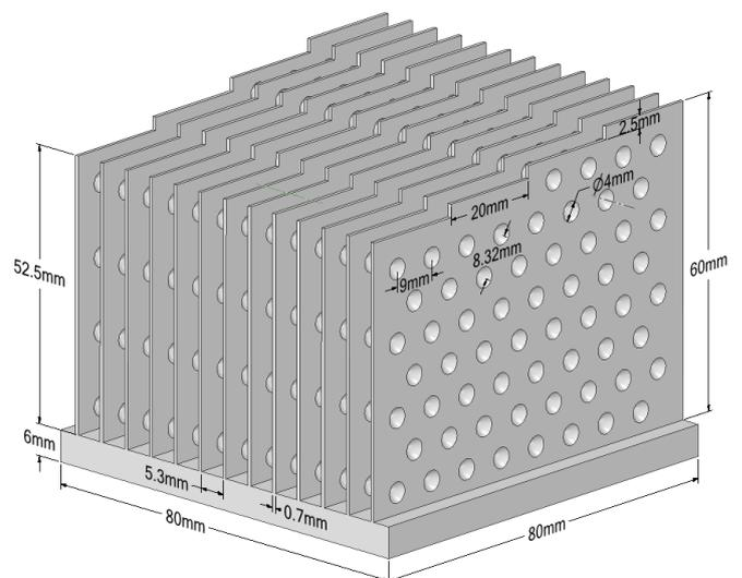
Figure 3: Stepped flat plate HS with staggered dimples
