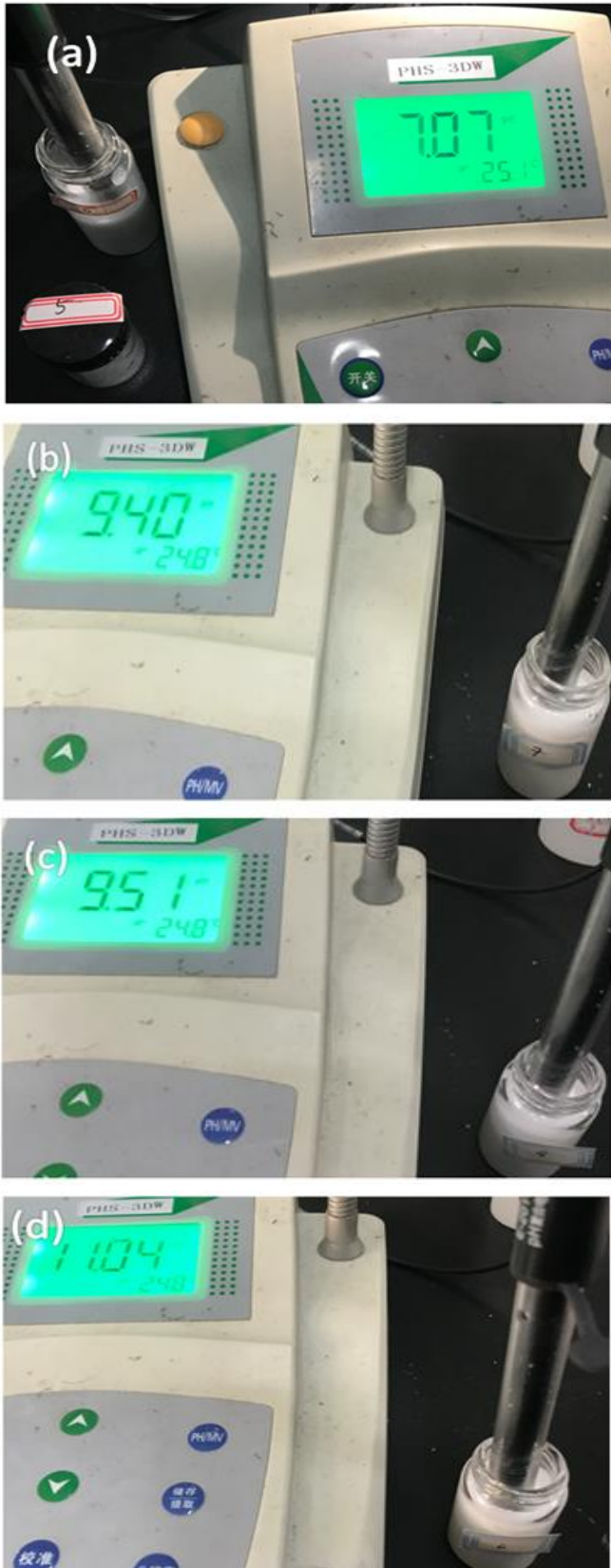
Figure S1: pH measurement of (a) Unmodified \text{TiO}_2 , and \text{TiO}_2 particles modified with (b) \text{NaHCO}_3 , (c) \text{Na}_2\text{CO}_3 and (d) \text{NaOH} .
